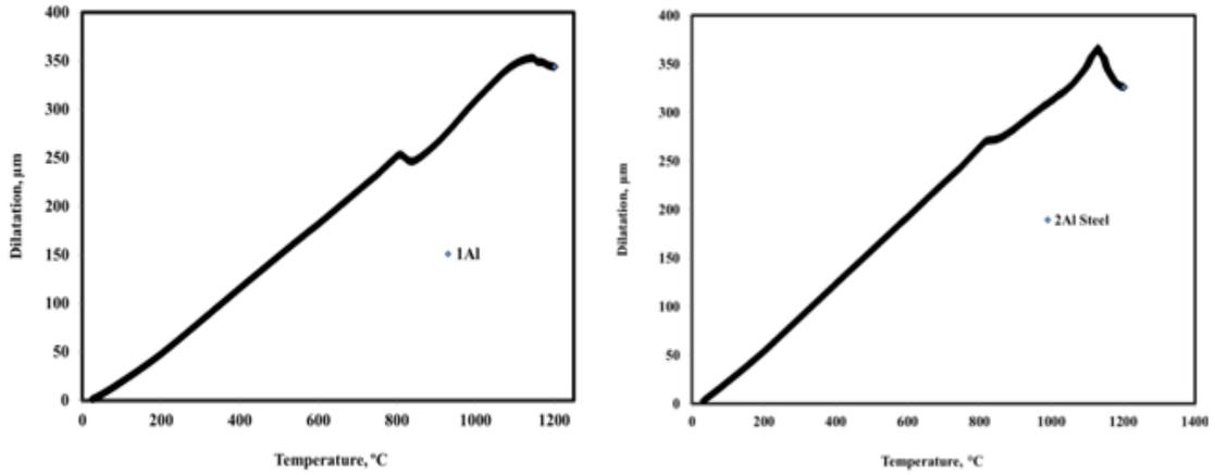
Figure 2: Total Dilatation Behavior of Alloy 1 and Alloy 2
