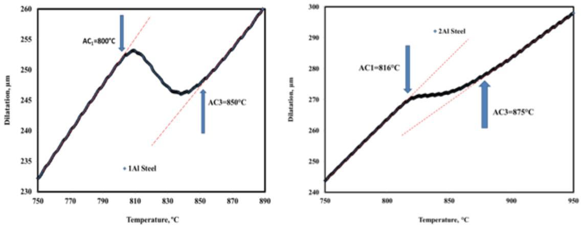
Figure 3: Critical Transformation Temperature AC1 and AC3
